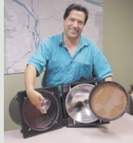
Paul Zebell, signal operations specialist, holds an incandescent bulb and an LED replacement module.
