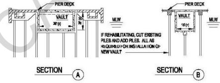
STRUCTURAL MODIFICATIONS/NEW FOR ELECTRICAL VAULT
