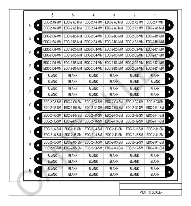
Figure 3-24 Pier Fiber Distribution Center EDC 1 Front Detail Submarine Pier
