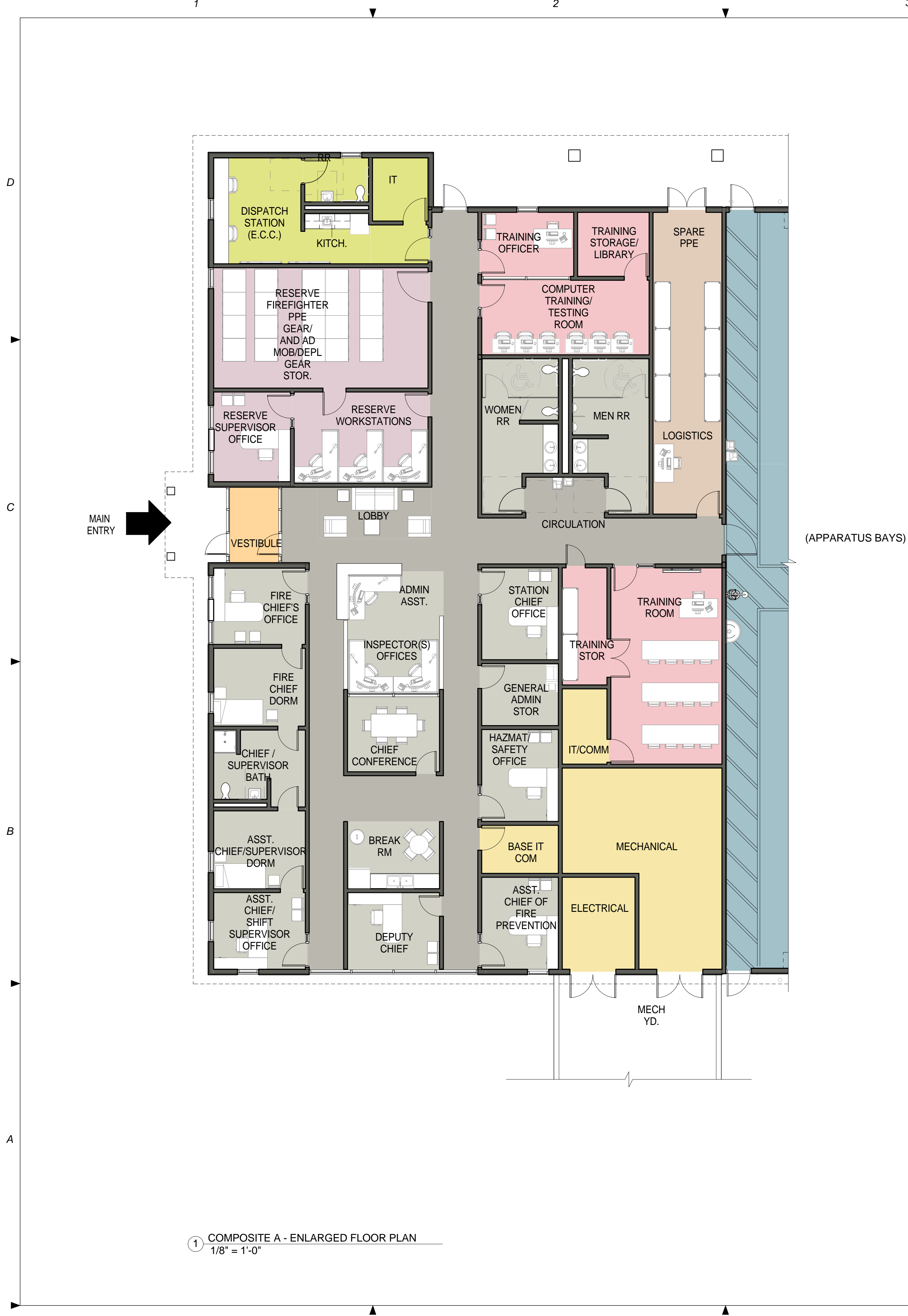
2 COMPOSITE A - ENLARGED FLOOR PLAN 1/8" = 1'-0"
