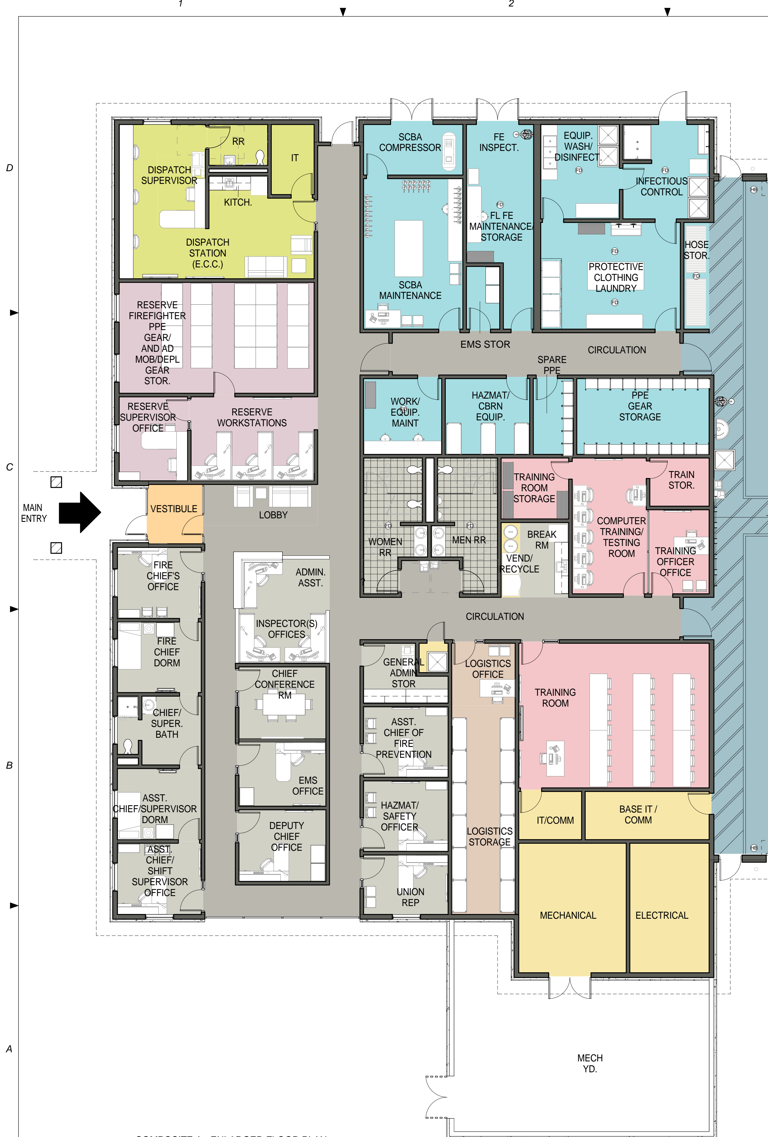
1 COMPOSITE A - ENLARGED FLOOR PLAN 1/8" = 1'-0"
